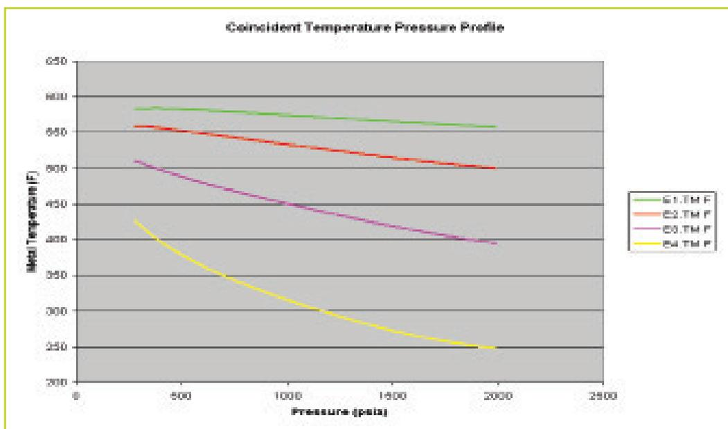
Figure 3: Coincident Temperature and Pressure Profile
