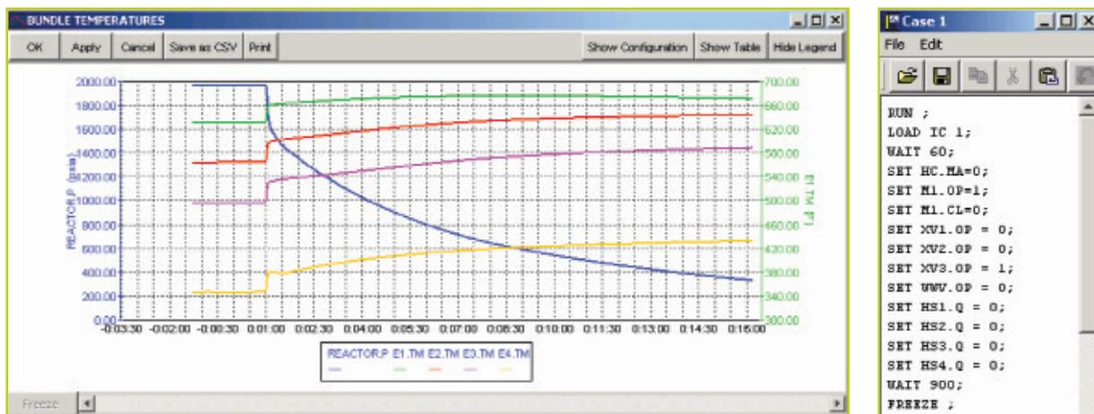
Figure 2: Reactor Pressure and Effluent Exchanger Temperatures
