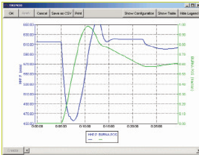
Figure 3: HP Steam Pressure (Blue) and Supplemental Firing Response (Green) without supplemental firing feed forward control signal
