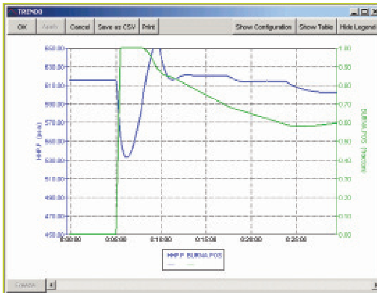
Figure 4: HP Steam Pressure (Blue) and Supplemental Firing Response (Green) with supplemental firing feed forward control signal
