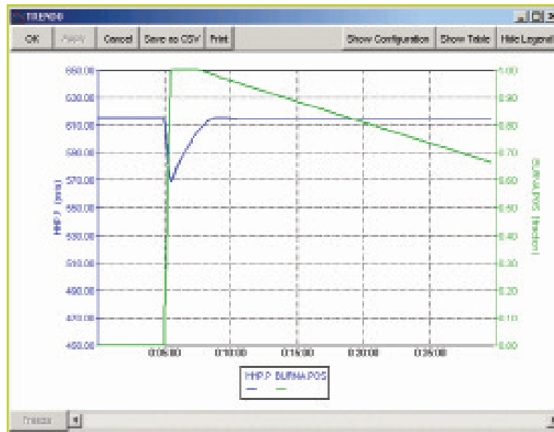
Figure 5: HP Steam Pressure (Blue) and Supplemental Firing Response (Green) with supplemental firing feed forward control signal and trip of condensing steam turbine
