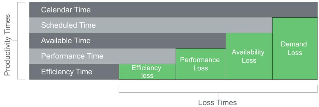
Note: The Time Loss Accounting Model may vary from company to company according to the different standards employed. This will not affect the ability of the system to measure Real-Time OEE as long as the outcome provides a means to measure OEE as a benchmark that can be used for continuous improvement.
