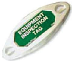
The Wonderware ST-1 RFID tag is a ruggedized tag that provides a permanent, durable, and cost-effective method for asset identification and control. Since the ST-1 tag is read by radio waves instead of light waves, as with bar codes, it will communicate through non-metallic materials such as paint, plastic, grease, dirt; and is impervious to vibration, light, water, and heat (up to 100°C).
